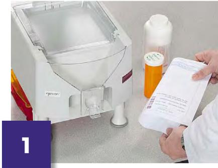
**Scan Label** – Scan barcode containing NDC, quantity, and Rx number.
