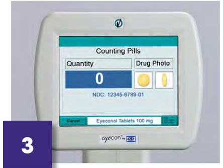
**Verify** – Eyecon will proceed to count mode if Rx label matches the stock bottle. Eyecon will display error if mismatch is detected.
