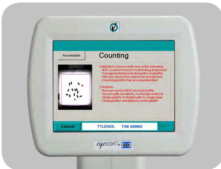
The highlighted shadow images represented on the left side of the display illustrate the location of the pill fragments or foreign matter on the counting platter.
