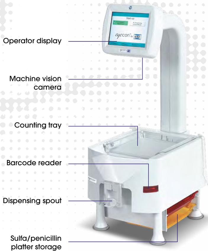
The Eyecon is a unique machine vision counting system. A camera mounted above the counting platter captures photo images used to count pills five times per second. Foreign matter and pill fragments that vary significantly from the reference image are easily identified on the counting platter. The operator is alerted to the presence of this foreign matter, ensuring the quality of prescriptions filled on the Eyecon.
