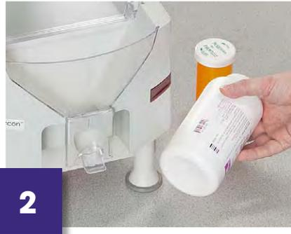
**Scan Bottle** – Scan barcode on stock bottle to validate that you've pulled the correct medication.
