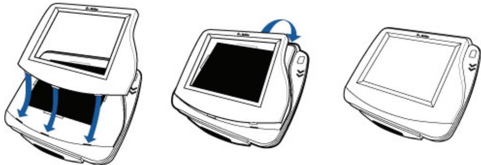
**Figure 11** Installing the Trimplate
