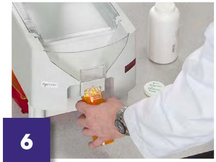
**Fill Vial** – Use vial to lift funnel gate and allow pills to flow into vial.
